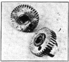
Check you fit right type of cam: upper version has flat rear face, part on right is shouldered.
