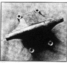
Alloy casting linking rear of engine to frame comes from post-'70 Meteors.
